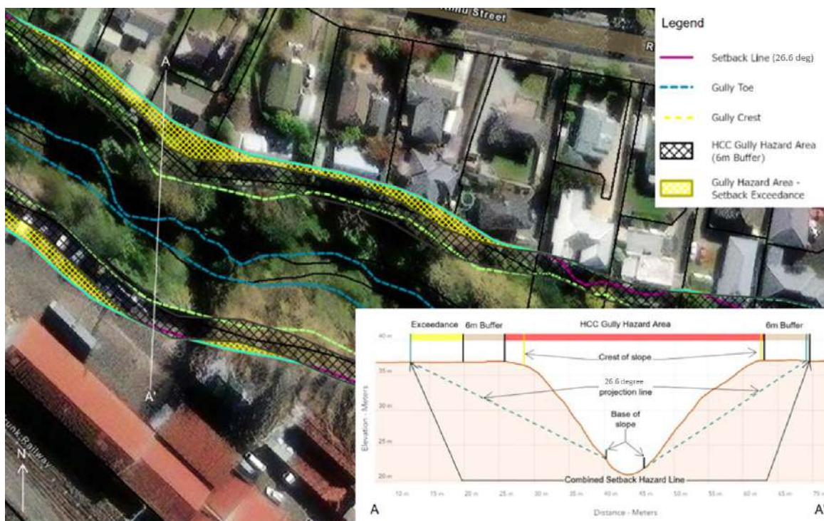
Figure 7.6: Gully setback analysis results; detail near Main Trunk railway, Waitawhiriwhiri Gully (T+T Slope, 2024).
